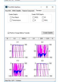
13. If your DUT is an active component, click the **Transistor** tab. This allows you to plot some figures of merit (FOMs) for the component:
